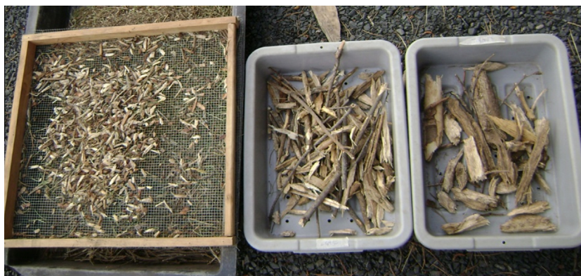
Fig. 2. Masticated fuel beds typically include a mixture of size classes with many irregularly shaped pieces. Here, masticated fuel particles taken from a mixed-conifer stand in northern Idaho are sorted into 1-h, 10-h, and 100-h size classes (left to right respectively). Fuels were removed from the field 2 weeks following mastication. Note the irregular particle shapes and abundance of small diameter particles relative to logging slash.
